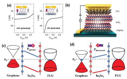
Fig. 3 (a) Schematic diagram of ferroelectric adjustable diode structure. (b) I-V curve of diode rectification function. (c and d) Explanation of the switchable rectification behaviour of a ferroelectric diode, showing the energy band diagram of the graphene/In<sub>2</sub>Se<sub>3</sub> heterostructure and the evolution of the Schottky barrier in the ferroelectric polarization reversal. (Reproduced from ref. 40 with permission from The Royal Society of Chemistry.)
