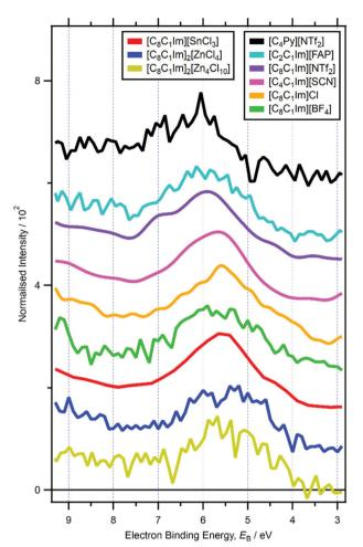
Fig. 4 Subtracted RXP spectra for  $N_{cation}$  for nine ionic liquids ( $h\nu \sim 402 \, \text{eV}$ ). These RXPS traces were produced by subtraction of resonant XP spectrum minus non-resonant XP spectrum using the procedure outlined in ref. 48. All electron spectra were charge referenced using methods outlined in Section 2.4.
