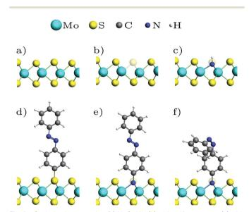
Fig. 1 Optimized geometries: (a)  $MoS_2$  ML, (b) with sulfur vacancy, (c) with NH, (d) with *trans*-azobenzene (AB), (e) with *trans*-aminoazobenzene (AAB), (f) with *cis*-AAB in the vacancy. Note that the systems are fully periodic, for a top view see *e.g.* Fig. 3a.
