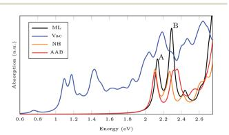
Fig. 6 Exciton absorption spectrum (GdW/BSE) of pristine MoS<sub>2</sub> monolayer (ML), with sulfur vacancy (Vac), NH and trans-aminoazobenzene (AAB) in a vacancy
