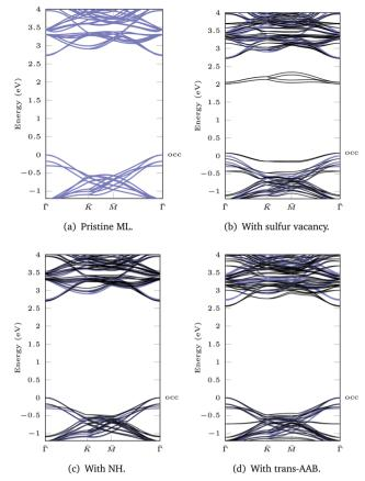
Fig. 5 LDA+GdW band structures for  $3 \times 3$  supercells. The pristine ML is shown in blue. The valence band maximum of the ML is set to 0 eV to allow for better comparison. The highest occupied (occ) band of the functionalized system is labeled.
