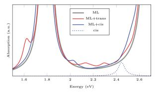
Fig. 8 TDDFT spectra of pristine ML, and of MLs functionalized with AAB in trans and cis configuration. Absorption of isolated cis-AAB is shown for comparison, trans-AAB is not shown, as the excitation at 2.32 eV has very small oscillator strength.
