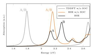
Fig. 7 Absorption spectra calculated using GdW/BSE and TDDFT. The splitting into A and B exciton is due to spin-orbit coupling (SOC).
