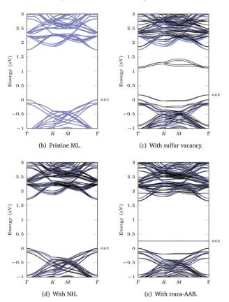
Fig. 3 (a) Geometry of a  $3 \times 3$  supercell (with *cis*-AAB as an example) and the corresponding 2D Brillouin zone (BZ). (b)-(e) LDA band structures are calculated between the points of high symmetry (blue path in the BZ). The band structure of pristine ML is shown in blue. The valence band maximum of the ML is set to 0 eV to allow for better comparison. The highest occupied (occ) band of the functionalized system is labeled.
