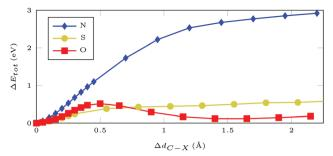
Fig. 2 Total DFT energy differences for a  $5 \times 5 \text{ MoS}_2$  supercell with AB attached at an atom of type X = (N/S/O) filling a sulfur vacancy. Geometries were optimized with restrained C-X distance.
