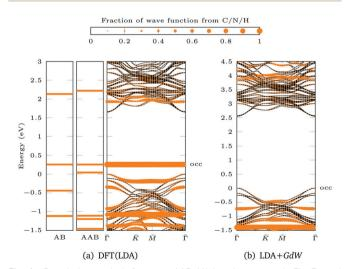
Fig. 4 Population analysis for trans-AAB-ML bandstructures in Fig. 3e and 5d: the size of the orange points is proportional to the part of the wave function stemming from C/N/H atoms. The valence band maximum of the ML is set to 0 eV. The highest occupied (occ) band of the functionalized system is labeled. (a) LDA band structures of AB (left), AAB (center) and trans-AAB-ML (right). (b) LDA+GdW band structures of trans-AAB-ML. Note the different energy scales.
