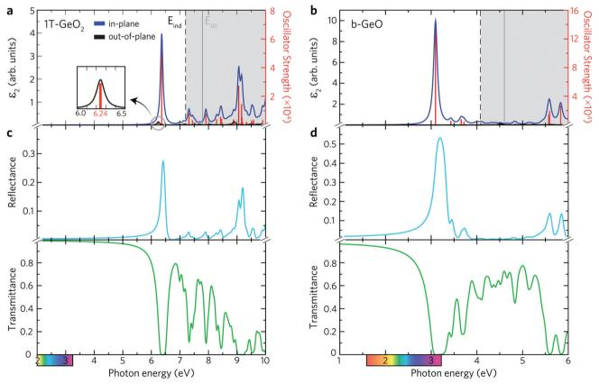
Fig. 3 For 1T-GeO<sub>2</sub> and b-GeO single-layers, (a and b) the calculated in-plane and out-of-plane components of the imaginary parts of the dielectric functions, (c and d) reflectance, and transmittance spectra, as a function of photon energy. Vertical red lines stand for oscillator strengths of optical transitions, while black dashed and grey solid lines mark the positions of indirect and direct band gaps of the crystals, respectively
