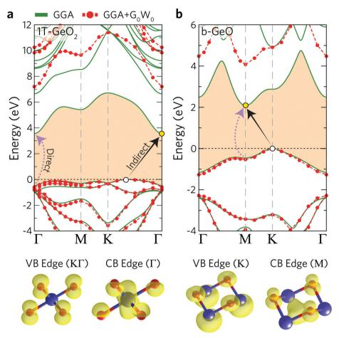
Fig. 2 Calculated GGA (green solid) and quasiparticle (GGA + G<sub>0</sub>W<sub>0</sub>, red dashed curves) electronic band structures (top panel), and the illustrations of atomic orbitals contributing to the VBM and CBM edges (bottom panel) for (a) 1T-GeO2 and (b) b-GeO single-layers. VBM and CBM edges are marked with white and yellow dots, respectively.
