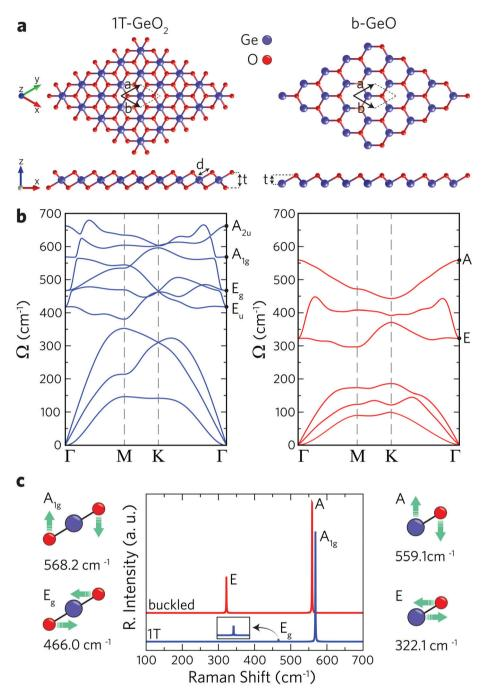
Fig. 1 The optimized structures of single-layer 1T-GeO<sub>2</sub> and b-GeO. (a) Top and side views (left panel for 1T-GeO<sub>2</sub> and right panel for b-GeO), (b) phonon band structures in the same order, and (c) the corresponding Raman activity of zone-centered phonon vibrations. Atomic vibrations of atoms for the four Raman active modes.
