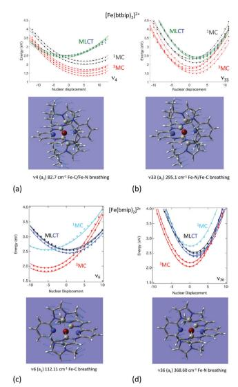
Fig. 2 Cuts of the diabatic potential energy surfaces as a function of the nuclear displacements associated with the dominant normal modes in  $[Fe(bmip)_2]^{2+}$  (bottom) and  $[Fe(btbip)^2]^{2+}$  (top). (Adapted from ref. 57b and 79 with the permission of the American Chemical Society).
