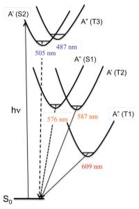
Scheme 6 Schematic representation of the potential energy curves associated with the low-lying excited states of [Re(Br)(CO)<sub>3</sub>(bpy)].
