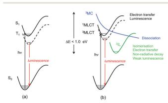
Scheme 1 (a) Luminescence decay based on the two-state model. (b) Cartoon of the typical radiative and non-radiative decays in coordination
