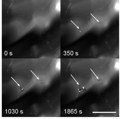
Fig. 3 Images of crystal growth of NaBr (AH) from an aqueous supersaturated solution following NPLIN. Solution conditions: C = 11.5 mol kg<sup>-1</sup>, T= 21 °C, S = 1.29 (DH) or 1.02 (AH). The crystals were imaged through the bottom of the vial and are shown between 0 and 31 minutes after the laser pulse (1064 nm). Crystals were first visible approximately 25 s after the laser pulse. Scale bar represents 2 mm.
