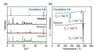
**Fig. 6** (a) PXRD patterns and (b) DSC thermograms for the crystalline and ground samples of  $1-\beta$ . The  $T_p$  and  $T_m$  values are noted near the corresponding peaks.
