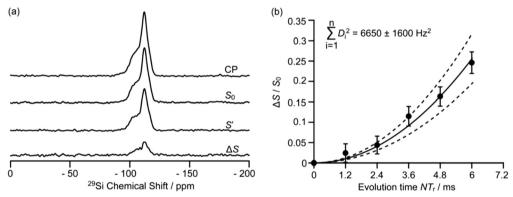
Fig. 12 (a)  $^{29}$ Si CP,  $^{29}$ Si CP spin echo ( $S_0$ ), and  $^{29}$ Si  $\{^{13}$ C} REDOR signal reintroducing dipolar couplings (S') and the difference  $\Delta S$  signal ( $S_0 - S'$ ) at a MAS rate of  $v_r = 5$  kHz for H-ZSM-5 zeolite. (b) Plot of the REDOR fraction  $S_0 - S'/S_0$  as a function of evolution time  $N/v_r$  and corresponding bestfit curve (black line) and fit boundaries (dashed lines). Ref. 72 - published by the Royal Society of Chemistry.
