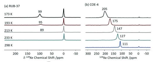
Fig. 8 Variable temperature hyperpolarised static <sup>129</sup>Xe NMR spectra of (a) RUB-37 and (b) COE-4. Reprinted from ref. 63: structural investigation of interlayer-expanded zeolite by hyperpolarized <sup>129</sup>Xe and <sup>1</sup>H NMR spectroscopy, 109555, Copyright 2019, with permission from Elsevier.
