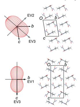
Fig. 6 Thermal expansion tensors and orientation of the principal expansion axes in FII (top) and FIII (bottom). The expansion coefficients along each axis are indicated in Table 2. The third principal axis is approximately perpendicular to the page. The axis directions are averaged over the temperature range 100–300 K.
