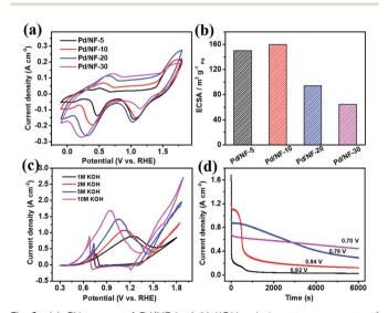
**Fig. 2** (a) CV curves of Pd/NF in 1 M KOH solution at a scan rate of 10 mV s $^{-1}$ ; (b) corresponding ECSA values of Pd/NF; (c) CV curves of Pd/NF-10 in alkaline EG solution (different concentrations of KOH + 1 M EG) at a scan rate of 10 mV s $^{-1}$ ; (d) chronoamperometry curves of Pd/NF-10 in alkaline EG solution (10 M KOH +1 M EG) under different potentials.
