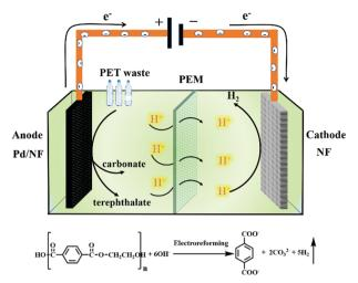
Scheme 1 Schematic illustration of the electroreforming of PET into high value-added chemicals and  $\rm H_2$  fuel.
