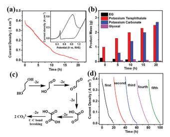
Fig. 3 (a) PET electro-reforming chronoamperometry curve on Pd/NF-10 at 0.7 V vs. RHE; inset: CV curve of the PET electroreforming substrate at a scan rate of 10 mV s $^{-1}$ ; (b) product analysis of PET electroreforming on Pd/NF-10 at 0.7 V vs. RHE; (c) proposed reaction mechanism for EG oxidation on the Pd/NF-10 electrocatalyst; (d) stability test for PET electro-reforming on Pd/NF-10 at 0.7 V vs. RHE for 5 cycles.
