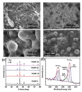
Fig. 1 SEM images of (a) Pd/NF-5, (b) Pd/NF-10, (c) Pd/NF-20, and (d) Pd/NF-30; (e) XRD patterns of Pd/NF; and (f) Pd 3d XPS spectrum of Pd/NF-10.
