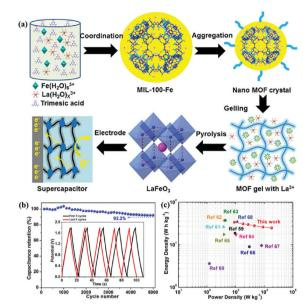
Fig. 5 (a) Schematic illustrations showing the synthesis of perovskite LaFeO<sub>3</sub>. (b) Cycling stability versus cycle number graph, inset: the first and last five GCD cycles. (c) Ragone plots (energy density vs. power density) of this work and other devices. Reproduced from ref. 61 with permission from Elsevier B.V., copyright 2020.
