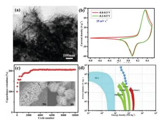
**Fig. 9** (a) TEM images of LSM15@NC scratched down from the Ni foam. (b) Comparative CV curves at a scan rate of 25 mV s $^{-1}$  within different potential windows of -0.8 to 0.5 V and -0.2 to 0.5 V. (c) Cycling performance (the insets show the morphology of LSM15@NC after 10 000 cycles). (d) Ragone plot. Reproduced from ref. 113 with permission from Elsevier B.V., copyright 2018.
