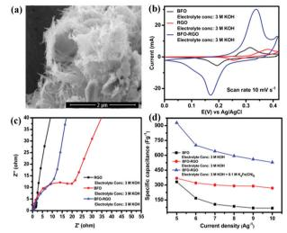
**Fig. 10** FESEM micrographs of (a) BFO. (b) Cyclic voltammetry curves of BFO, RGO, and BFO–RGO electrodes at a scan rate of 10 mV s $^{-1}$  in a 3 M KOH electrolyte. (c) Electrochemical impedance spectra of RGO, BFO, and BFO–RGO electrodes in a 3 M KOH electrolyte. (d) Change of the specific capacitance of BFO and BFO–RGO electrodes with changing current density from 5 to 10 A g $^{-1}$ . Reproduced from ref. 117 with permission from American Chemical Society, copyright 2018.
