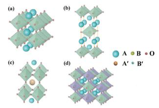
**Fig. 3** Crystal structure of (a) the ideal  $ABO_3$ -type perovskite oxides, (b) Ruddlesden–Popper perovskite oxides ((AO)( $ABO_3$ )<sub>n</sub>), (c) A-site ordered double perovskite oxides ( $AA'B_2O_6$ ) and (d) B-site ordered double perovskite oxides ( $A_2BB'O_6$ ).
