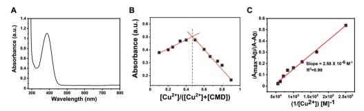
Fig. 2 UV-Vis characterization of metal-ligand binding: (A) UV-Vis spectra of the molecule ( $2 \times 10^{-5}$  M) with an absorption maximum centered at 387 nm. (B) Job's plot indicates that the ligand-to-metal binding ratio is 1:1 (number of experiments = 3). (C) The Benesi-Hildebrand plot provides a binding constant of the complexation  $(3.51 \times 10^5 \text{ M}^{-1})$  (number of experiments = 3).
