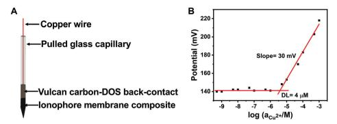
Fig. 5 Potentiometric characterization of the  $Cu^{2+}$  ISE: (A) schematic of the carbon-packed Cu(II) microsensor. (B) Potentiometric calibration of  $Cu^{2+}$  with the carbon-packed sensor. DOS: dioctyl sebacate. The sensors showed Nernstian slope of  $29.3 \pm 2.9$  mV/log [ $a_{Cu}^{2+}$ ] and detection limits of 3.5 + 1.0  $\mu$ M (number of experiments = 6).
