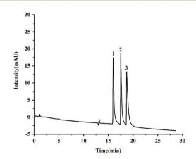
Fig. 6 Separation behavior of amino acids on the TzDa@capillary. Experimental conditions: mobile phase, 40% methanol in pH 8.0 20 mM phosphate buffer; applied voltage, 20 kV; injection, 25 mbar × 5 s; detection wavelength, 210 nm. Peaks: 1, tryptophan; 2, tyrosine; 3, phenylalanine.
