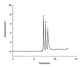
Fig. 4 Separation behavior of phenolic compounds on TzDa@capillary, Experimental conditions; mobile phase, 25% ACN in pH 9.0 30 mM phosphate buffer; applied voltage, 20 kV; injection, 7 mbar × 5 s; detection wavelength, 230 nm. Peaks: 1, hydroquinone; 2, resorcinol; 3, catechol.
