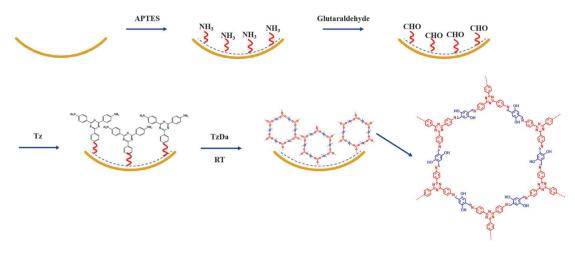
Fig. 1 Schematic procedure for the fabrication of the TzDa@capillary.
