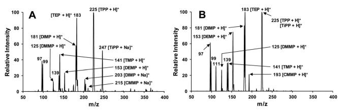
Fig. 3 3D-PCSI-MS collected on the portable AI-MS from a mixture of DMMP, TMP, DEMP, DIMP, TEP, CMMP, TPP, and TiPP (all at 5 ppm each) in sand. Spectra (A) collected at 1 min of analysis time yield both protonated and sodiated adducts for some target CWA simulants, where spectra (B) from ~7 min predominately show only the protonated forms, as salt leaves the sand matrix.
