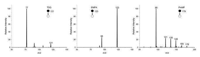
Fig. 2 MS/MS spectra for CWA hydrolysis products at their respective empirical LODs on the benchtop ion trap instrument. The [M - H] peak was isolated and fragmented in MS<sup>2</sup> for all CWA hydrolysis products.
