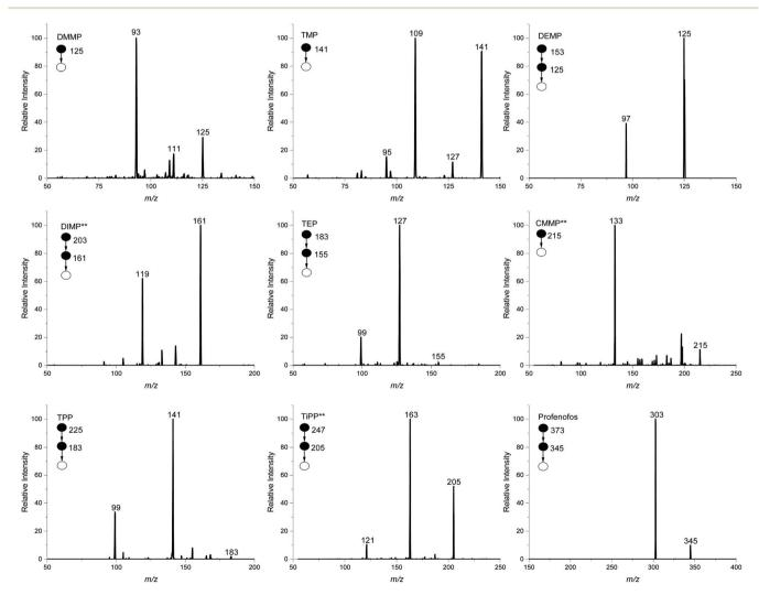
Fig. 1  $MS^n$  spectra of CWA simulants at their respective empirical LODs on the benchtop ion trap instrument. The  $[M + H]^+$  peak was isolated for all CWA simulants except DIMP, CMMP, and TiPP which the sodium adduct  $[M + Na]^+$  was isolated and fragmented. The use of the sodium adduct is indicated by \*\* next to the compound name.
