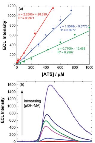
Fig. 3 (a) Typical trend of maximum ECL signal against [ATS] at pH 9.0 for MA (red squares), AMP (green circles) and pOH-MA (blue triangles). (b) Typically, ECL response for increasing [pOH-MA] in 0.1 M PBS at pH 9.0 scanned over the potential range  $0.8 \le E \le 1.6 \text{ V}$  vs. Ag/AgCl at a scan rate of 100 mV s<sup>-1</sup>. PMT was biased at 650 V (error bars represent standard deviation obtained from triplicate results).
