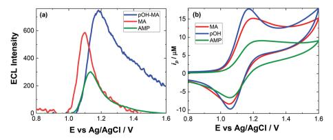
Fig. 1 (a) Typical ECL response and (b) typical CV for 500 μM pOH-MA (blue), 500 μM AMP (green) and 500 μM MA (red) in 0.1 M PBS, pH 9. Scanned over the potential range  $0.8 \le E \le 1.6 \text{ V}$  vs. Ag/AgCl at a scan rate of 100 mV s<sup>-1</sup>. PMT was biased at 650 V.
