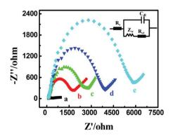
Fig. 2 EIS characterization of the different electrodes in 0.1 M KCl containing 5 mM [Fe(CN)<sub>6</sub>]<sup>3-/4-</sup>: (a) bare Au electrode, (b) Fc-H1/Au electrode, (c) MCH/Fc-H1/Au electrode, (d) probe STP/MCH/Fc-H1/Au electrode, (e) MB-H2/probe STP/MCH/Fc-H1/Au electrode.
