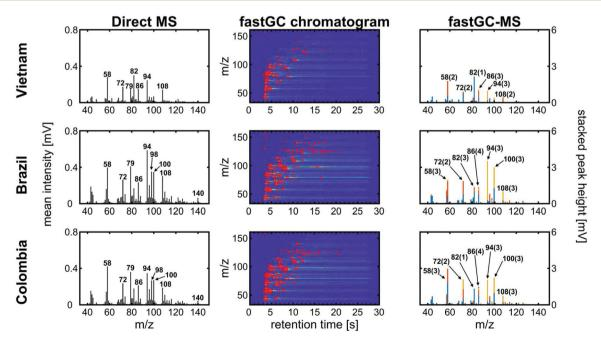
Fig. 5 The averaged SPI mass spectra (left column), chromatogram with peak heights highlighted as bubbles (centre column) and SPI mass spectra with stacked intensities from individual peak picking (right column) for Vietnam Robusta, Brazil Arabica and Colombia Arabica ground coffees from the same roast profile. The numbers in the mass spectra refer to the m/z and the number in the brackets to the number of individual peaks detected at a nominal m/z.
