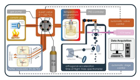
Fig. 1 Schematic setup of the fastGC-SPI-TOFMS system in "sampling" mode for the headspace analysis of needles with a sampling unit, a 6-port-2-way valve for changing to helium as the GC carrier gas, an electrical modulator, an optically heated fastGC, a VUV lamp for SPI and an orthogonal-acceleration TOFMS
