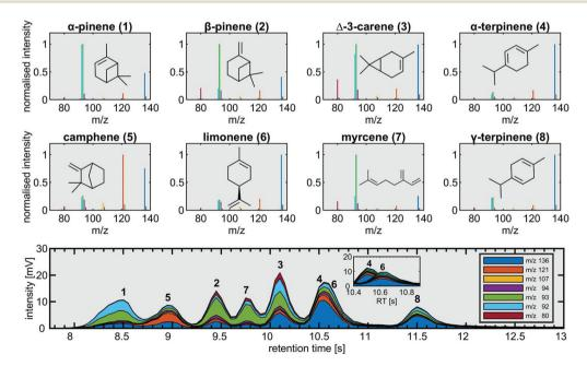
Fig. 4 SPI mass spectra of eight individual monoterpenes (top) and the chromatogram of the monoterpene mixture (bottom). The overlapping peaks of  $\alpha$ -terpinene (4) and limonene (6) are deconvolved by non-negative matrix factorization (NMF) due to slight differences in fragmentation with monoterpene-related fragments highlighted in colours.
