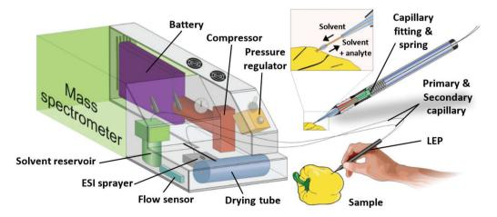
Fig. 1 Scheme of the portable ESI source with its major components and the handheld LEP.
