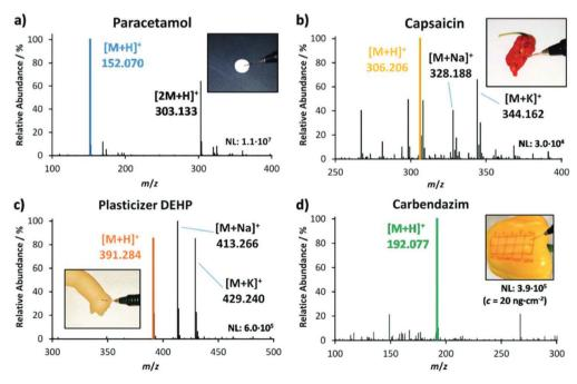
Fig. 2 Mass spectra of various analytes measured directly from the sample object with the self-sustaining LEP source attached to an orbital-trapping mass spectrometer. (a) Paracetamol pill, (b) capsaicin from a dried chili pepper 'Carolina Reaper', (c) plasticizer DEHP from a toy puppet and (d) carbendazim from a fresh pepper.
