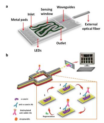
Fig. 1 (a) Schematic of the chip with the fluidic on top and the positioning of the external optical fiber used for the collection of the transmitted spectra of the integrated on chip MZIs. (b) Schematic of a single MZI and of the immunoassay steps for detection of bovine  $\kappa$ -casein in buffalo mozzarella and feta cheese.
