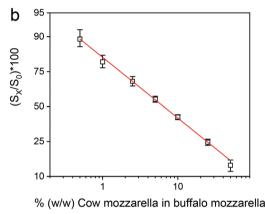
Fig. 6 (a) Net real-time signal responses obtained for cow cheese calibrators (0-50%, w/w) in the mozzarella cheese matrix. (b) Typical calibration curve obtained for mozzarella cheese adulteration with cow cheese. Each point is the mean value of 3 measurements + SD.
