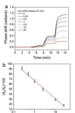
Fig. 7 (a) Net real-time signal responses obtained for cow cheese calibrators (0–25%, w/w) in the feta cheese matrix. (b) Typical calibration curve obtained for feta cheese adulteration with cow cheese. Each point is the mean value of 3 measurements  $\pm$  SD.
