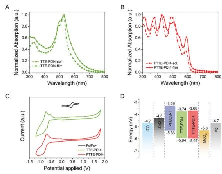
Fig. 2 Normalized absorption spectra of (A) TTE-PDI4 and (B) FTTE-PDI4 in chloroform solution (10<sup>-5</sup> M) and as pristine films. (C) Cyclic voltammetry curves of TTE-PDI4 and FTTE-PDI4 films. (D) Energy level diagram of the OPV device.
