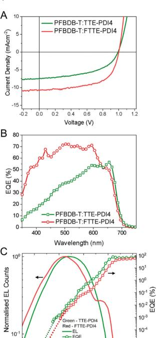
Fig. 3 J-V curves (A) and EQEs (B) for the optimized devices based on the PFBDB-T:TTE-PDI4 and PFBDB-T:FTTE-PDI4 blends. (C) Electroluminescence (solid lines), external quantum efficiency (line and symbols), and extended external quantum efficiency (symbols) calculated using reciprocity from the EL spectra of PFBDB-T:TTE-PDI4 (green) and PFBDB-T:FTTE-PDI4 (red) blend devices.
