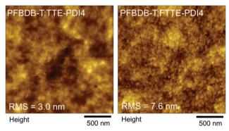
Fig. 4  $\,$  AFM height images (2  $\mu m \times 2~\mu m)$  of the PFBDB-T:TTE-PDI4 (left) and PFBDB-T:FTTBPDI4 (right) blend films. The topographical height difference ( $\Delta z$ ) are 21 nm and 51 nm, respectively.
