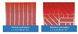
Fig. 12 Schematic illustrations of vertically and randomly oriented BA2MA3Pb4l13 crystal orientations that lead to different thermal conductivities. Reprinted with permission from ref. 32. Copyright (2020) American Chemical Society
