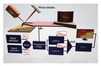
Fig. 6 Schematic illustration of extended quantitative thermal conductivity measurements by SThM applying the so-called 3ω-technique in the frequency domain. Reprinted with permission from ref. 50. Copyright (2019) American Chemical Society.
