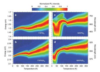
Fig. 9 Temperature dependence of normalized steady-state PL on (a) FAPbl<sub>3</sub>, (b) FAPbBr<sub>3</sub>, (c) MAPbl<sub>3</sub>, and (d) MAPbBr<sub>3</sub>. From ref. 156. Reprinted with permission from Springer Nature.
