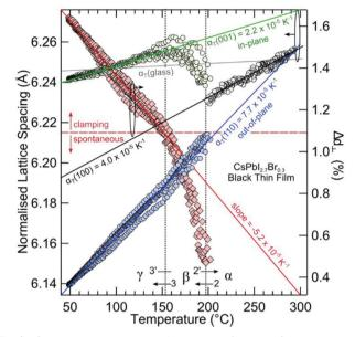
Fig. 8 Structural phase kinetics of strained  $\alpha$ -,  $\beta$ -, and  $\gamma$ -CsPbl<sub>3</sub> perovskite thin films. From ref. 138. Reprinted with permission from AAAS.
