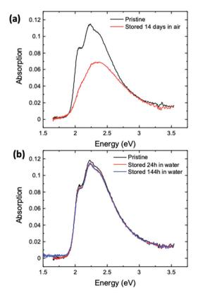
Fig. 8 Evolution of absorption spectra for P3HT films stored in air (a) or immersed in water (b).
