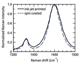
Fig. 6 Comparison of the resonant Raman spectra (C-C and C=C modes) of ink-jet printed (solid black line) and spin-coated (blue dashed line) P3HT films, excited using a 488 nm laser.
