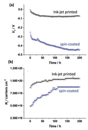
Fig. 4 (a) Ink-jet printed and spin-coated P3HT based EGOFETs' threshold voltage (a)  $V_T$ , and (b) total density of localized (trap) states  $N_t$  as extracted from the modelling of the transfer characteristics (see text for details)
