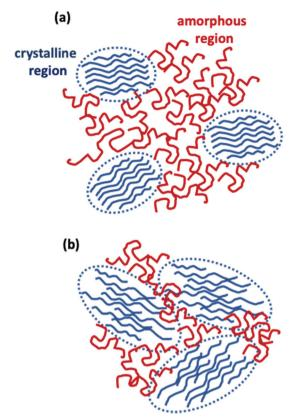
Fig. 7 Pictorial representation of the P3HT structure for ink-jet printed (a) and spin-coated (b) films. In the printed film smaller crystalline regions with better  $\pi - \pi$  stacking can be found. The spin-coated one has larger and more crystalline regions with overall worse  $\pi - \pi$  stacking features.
