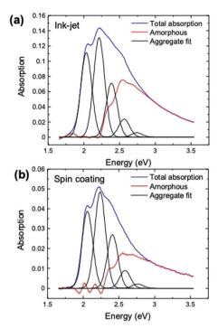
Fig. 5 Comparison of the absorption spectra of ink-jet printed (a) and spin-coated (b) P3HT films.
