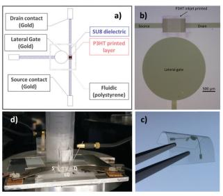
Fig. 1 (a) Schematic representation and (b) optical microscope image of an EGOFET fabricated by ink-jet printing and standard photolithography scale bar is 500  $\mu$ m; (c) picture of the device fabricated on a poly(ethylene 2,6-naphthalate) (PEN) flexible substrate; (d) picture of the device after a polystyrene cell is glued around the transistor channel, the cell is connected to a water reservoir visible in the back
