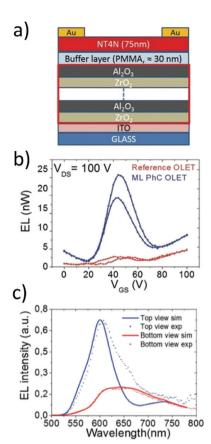
Fig. 17 (a) NT4N-based OLET including a multilayer photonic crystal (ML PhC); (b) electroluminescence of the ML PhC OLET as a function of  $V_{\rm GS}$  in comparison to that of a reference device; (c) electroluminescence spectra recorded from the top side and the bottom side of ML PhC OLETs. Adapted with license permission no. 4864750204768 from Natali *et al.*, Adv. Funct. Mater., 2017, 27, 1605164 and Wiley-VCH.
