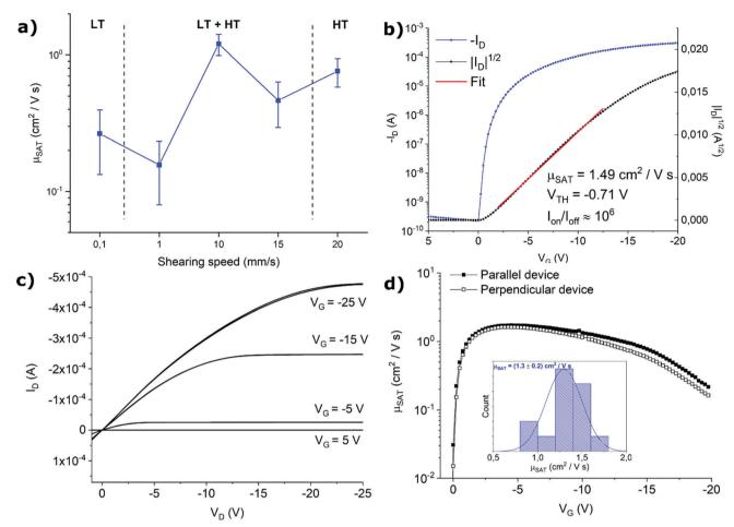
Fig. 4 (a) Mobility vs. shearing speed plot. Representative transfer (b) and output (c) characteristics for a diF-TES-ADT:PS film deposited at 10 mm s<sup>-1</sup>. (d) Mobility profiles for films coated with the channel parallel (filled squares) and perpendicular (empty squares) to the shearing direction (inset: device mobility statistics).
