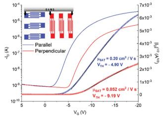
Fig. 5 Transfer characteristics of representative OFET devices with channel length parallel (blue line) and perpendicular (red line) with respect to the solution shearing direction, fabricated at  $1 \text{ mm s}^{-1}$ .
