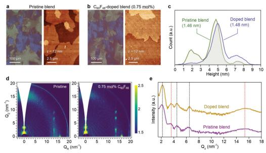
Fig. 4 (a and b) Polarized optical microscopy and atomic force microscopy images of pristine and p-doped C<sub>8</sub>-BTBT:C<sub>16</sub>IDT-BT layers processed via blade-coating. (c) Surface height histograms of the pristine and p-doped  $C_8$ -BTBT: $C_{16}$ IDT-BT layers extracted from the AFM images. (d) 2D GIWAXS images of the pristine and p-doped blend layers. (e) Plots of the integrated intensity versus Q (nm<sup>-1</sup>) for out-of-plane Bragg sheets taken from (d).
