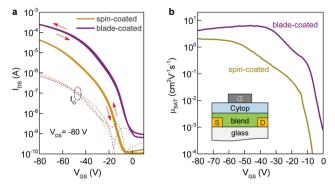
Fig. 3 (a) Transfer characteristics of spin-coated and blade-coated  $C_8$ -BTBT: $C_{16}$ IDT-BT OTFTs measured at  $V_{DS}$  = -80 V. Dotted lines represents the corresponding gate leakage  $(I_G)$  currents. The channel width and length of the devices were 1000 μm and 80 μm, respectively. (b) Hole mobility measured in saturation ( $\mu_{SAT}$ ) versus applied gate bias  $(V_{GS})$  for the C<sub>8</sub>-BTBT:C<sub>16</sub>IDT-BT-based OTFTs shown in (a).
