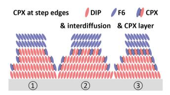
**Fig. 5** Schemes of possible mechanisms for CPX formation at the corrugated surface of a DIP film in the presence of F6. (1) CPX formation at step edges. (2) additional inter-diffusion of DIP and F6 at the very interface, and (3) possible formation of a CPX interlayer.
