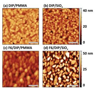
Fig. 3 Scanning force micrographs (2  $\times$  2  $\mu$ m<sup>2</sup>) for 25 nm DIP on PMMA/  $SiO_2/Si$  (a) and 30 nm DIP on  $SiO_x$  (b) as well as for 5 nm F6 on DIP/PMMA/ SiO<sub>2</sub>/Si (c) and 8.5 nm F6 on DIP/SiO<sub>x</sub>/Si (d). The grey bars indicate a length of 500 nm.
