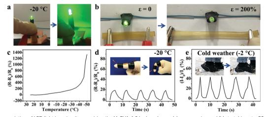
Fig. 9 Brightness variation of LED light in a circuit comprising the M-PVA-1.6 hydrogel upon (a) compression and (b) stretching at -20 °C. (c) Real-time relative resistance change of the anti-freezing M-PVA-1.6 hydrogel sensor during the cooling process. (d) Detection of finger bending at -20 °C. (e) Detection of treading behavior in cold weather.
