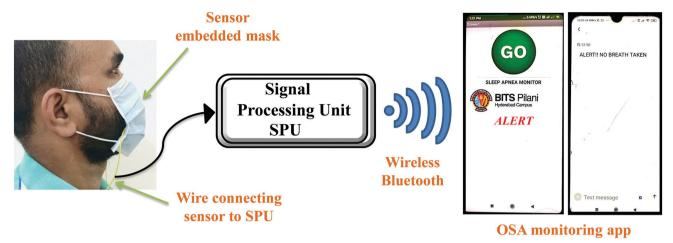
Schematic illustration of the face mask with the embedded HKUST-1-MoS<sub>2</sub> device showing real time operation using a smartphone device.
