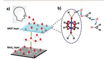
**Fig. 4** Breath sensing mechanism in the HKUST-1-MoS<sub>2</sub> integrated device. (a) Adsorption and transfer of water molecules from the MOF to the MoS<sub>2</sub> layer and (b) the mechanism of proton conduction in the MOF layer involving proton transfer from acidic water molecules coordinated to the metal cluster to the solvent molecules present in the channels. Only one cluster has been shown for clarity.
