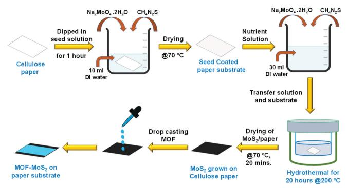
Scheme 2 Schematic illustration of growing MoS<sub>2</sub> on a cellulose paper substrate and dropcasting of MOF powder on the MoS<sub>2</sub> support for device fabrication.
