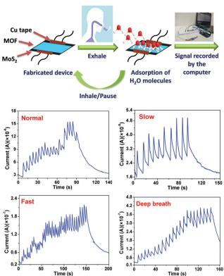
Fig. 3 (top) HKUST-1– $MoS_2$  fabricated sensor for breath sensing, and (bottom) breath sensing experiments showing variation in the current in response to different types of breaths: normal breath, slow breath, fast breath and deep breath.
