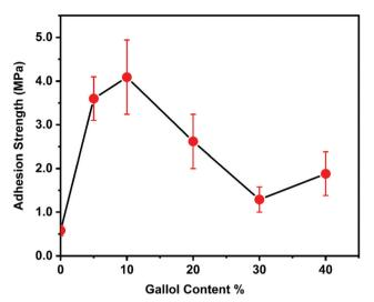
Fig. 3 Effect of gallol content on underwater adhesion strength. The error bars indicate standard deviation,  $n \ge 5$ .
