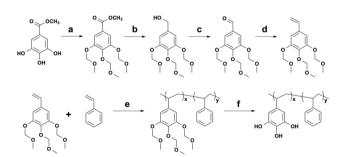
Scheme 1 Synthetic route of P(VGal-co-St). (a) DIEA, MOMCl, THF, 40 °C, 24 h. (b) LiAlH<sub>4</sub>, THF, 0 °C to r.t., 24 h. (c) MnO<sub>2</sub>, CH<sub>2</sub>Cl<sub>2</sub>, 24 h. (d) (Ph)<sub>3</sub>PCH<sub>3</sub>Br, t-BuOK, THF, 45 °C, 24 h. (e) AIBN, THF, 65 °C, 24 h. (f) HCl, MeOH, r.t., 24 h.
