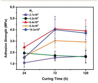
Fig. 1 Adhesion strength with different curing times. Error bars indicate standard deviation,  $n \ge 5$ .
