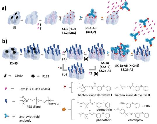
Scheme 1 Architecture and synthesis routes of the antibody-gated mesoporous materials (a) containing MCM-41 (S1) as mesoporous scaffold and (b) \$2-\$5 containing different types of SBA scaffolds (\$2: SBA-15, conventional long fibres; \$3: SBA-15 platelets; \$4: SBA-15 long fibres with enlarged pores; \$5: SBA-16 nanoparticles).
