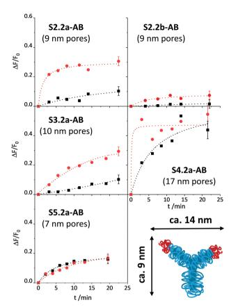
Fig. 7 Increase in fluorescence ( $\lambda_{\rm exc}$  = 532 nm;  $\lambda_{\rm em}$  = 550 nm) in the absence (black) and the presence (red) of 500  $\mu g\ kg^{-1}$  3-PBA for the supernatants of suspensions of the respective SBA materials as indicated in PBS buffer (80 mM, pH = 7.5, 10% iPrOH) as a function of time between analyte addition to the suspension and centrifugation of the suspension. The lines are included only as a guide to the eye for better illustration.
