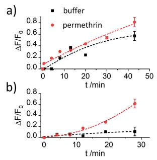
Fig. 4 Increase in fluorescence registered at 522 nm ( $\lambda_{exc}=490$  nm) in the presence (red) and the absence (black) of permethrin (6.6 mg kg $^{-1}$ ) for the supernatants of suspensions of two batches of materials **S1.1-AB** capped with antibody in (a) the absence and (b) the presence of BSA as blocking agent as a function of time between analyte addition to the suspension and centrifugation of the suspension. The lines are included only as a guide to the eye for better illustration.
