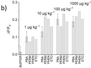
Fig. 8 (a) Increase in fluorescence because of SRG released from S2.2a-AB as a function of the concentration of 3-PBA (red) and permethrin (black) after 5 min of reaction; the lines exemplify four-parametric logistic fits. (b) Corresponding data in the presence of 3-PBA, permethrin, phenothrin and etofenprox.
