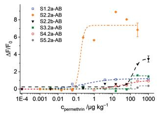
Fig. 9 Integrated density enhancement registered for the images taken with the 3D-printed holder and the smartphone as a function of the concentration of permethrin for the materials S1.2-AB, S2.2a-AB, S2.2b-AB, S3.2a-AB, S4.2a-AB, S5.2a-AB and S2.2b-AB; the lines exemplify fourparametric logistic fits.
