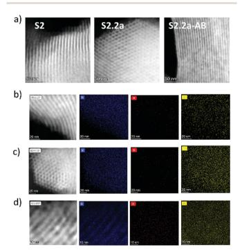
Fig. 3 (a) Scanning transmission electron micrographs of calcinated S2, S2.2a, and S2.2a-AB. (b)-(d) STEM images and corresponding EDX element maps of Si, S and C for (b) S2, (c) S2.2a and (d) S2.2a-AB
