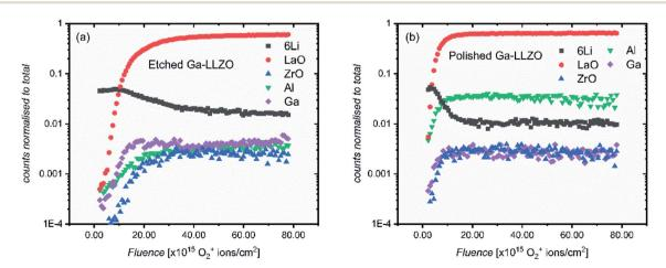
Fig. 4 ToF-SIMS depth profiles of etched (a) and polished (b) Ga-LLZO pellets, showing positive secondary ion species. The analysis was performed using 25 keV Bi<sup>+</sup> primary ions as the analytical beam and the sputtering was performed by 1 keV 300 nA  $O_2$ <sup>+</sup> beam (burst mode).
