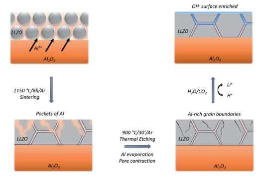
Fig. 9 Schematic of proposed processes occurring on a LLZO pellet during various thermal and atmospheric treatments, including: the formation of an Al-Li-O eutectic during sintering leading to Al diffusion in the grains and pore formation, Al evaporation and pore contraction during thermal etching and OH-enrichment of surfaces and grain boundaries upon reaction with CO2 and H2O, which is more acute on the activated, etched LLZO surface.
