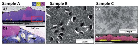
Fig. 8 Observation of  $SnS_x$  secondary phases in samples A, B and C. Sample A: STEM and EDX images, (a) with Cu (blue), Zn (pink) and Sn (yellow) and (b) close-up image of area marked with red rectangle. Sample B: (c) top view SEM with  $SnS_x$  flakes visible on surface. Sample C: (d) top view SEM with dendrite structures. (e) STEM and EDX image with Sn (yellow) and Zn (magenta).
