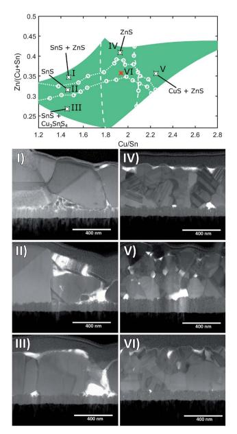
Fig. 6 Outline of sample A with boundaries for secondary phase regions. Bright field STEM images of samples extracted from positions as indicated in the map
