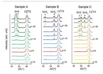
Fig. 4 XRD patterns of samples A, B and C in a  $2\theta$  range with expected SnS and SnS<sub>2</sub> reflections. y denotes the distance to the Cu/Sn = 2 line in mm.
