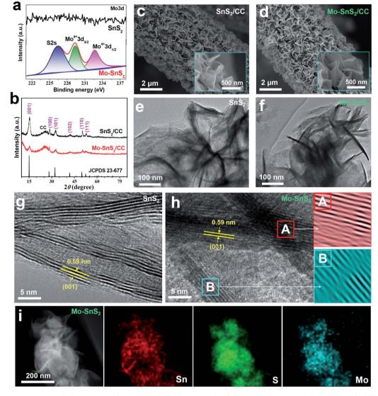
Fig. 1 (a) XPS Mo3d spectrum of  $SnS_2$  and Mo- $SnS_2$  nanosheets scraped from CC. (b) XRD patterns for  $SnS_2$ /CC and Mo- $SnS_2$ /CC. (c and d) SEM images of (c)  $SnS_2$ /CC and (d) Mo- $SnS_2$ /CC. (e and f) TEM images of (e)  $SnS_2$  and (f) Mo- $SnS_2$  nanosheets. (g and h) HRTEM images of (g)  $SnS_2$  and (h) Mo- $SnS_2$  nanosheets (A and B are the corresponding IFFT images recorded from regions A and B in (h)). (i) STEM element mapping images for Mo- $SnS_2$  nanosheets.
