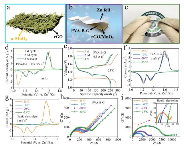
Fig. 3 (a) Graphic illustration of the rGO/MnO<sub>2</sub> nanocomposite. (b) Schematic diagram, (c) photograph, (d) CV curves of the initial three cycles at  $0.5 \text{ mV s}^{-1}$  at 25 °C, and (e) GCD curves of the initial three cycles at 0.5 A g<sup>-1</sup> at 25 °C of the PVA-B-G battery. (f and g) CV curves at 1 mV s<sup>-1</sup> and (h and i) Nyquist plots of (f and h) PVA-B-G battery and (q and i) liquid-electrolyte battery at different temperatures.
