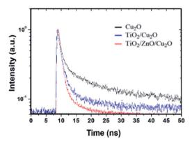
Fig. 5 Time-resolved PL spectra acquired with an excitation wavelength of 405 nm for the prepared Cu<sub>2</sub>O (black), TiO<sub>2</sub>/Cu<sub>2</sub>O (blue) and TiO<sub>2</sub>/ZnO/Cu<sub>2</sub>O (red) photoelectrodes.
