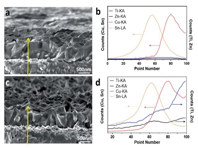
Fig. 2 Cross-section SEM images and corresponding line-scan profiles of (a and b) bare  $Cu_2O$  and (c and d)  $TiO_2/ZnO/Cu_2O$  photoelectrodes. The yellow arrow shows the scanning direction and the localised area where the SEM-EDS line-scan profiles were taken.
