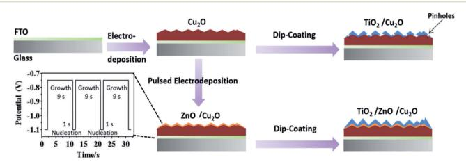
Scheme 1 Flowchart of the synthesis process for TiO<sub>2</sub>/Cu<sub>2</sub>O and TiO<sub>2</sub>/ZnO/Cu<sub>2</sub>O multilayered photoelectrodes.
