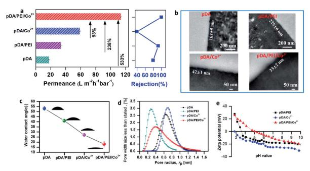
Fig. 2 (a) Permeance and (BTB) rejection results; (b) TEM images; (c) water contact angles (WCAs); (d) the pore size distribution; (e) zeta potentials of the binary (pDA/PEI and pDA/Co<sup>2+</sup>) and ternary (pDA/PEI/Co<sup>2+</sup>) coated membranes.
