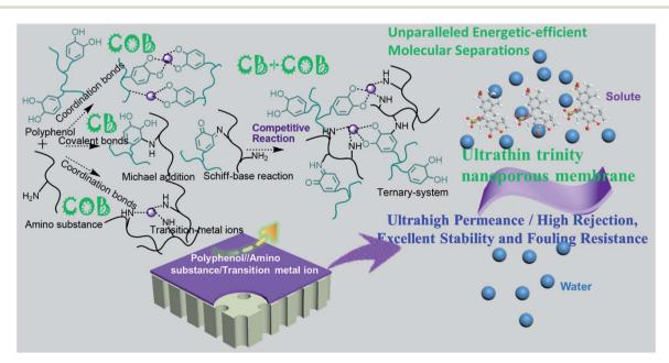
Fig. 1 The scheme of the fabrication process of the ultrathin trinity coating via CB/COB competitive reactions.
