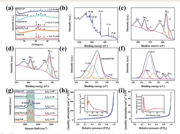
Fig. 3 (a) The XRD patterns, the XPS spectra of (b) the survey, (c) Ni 2p, (d) Co 2p, (e) O 1s and (f) P 2p for GO@NiCoP, (g) the Raman spectra, the N<sub>2</sub> adsorption-desorption isotherms and pore-size distribution (inset) of (h) GO@NiCoP and (i) NiCoP
