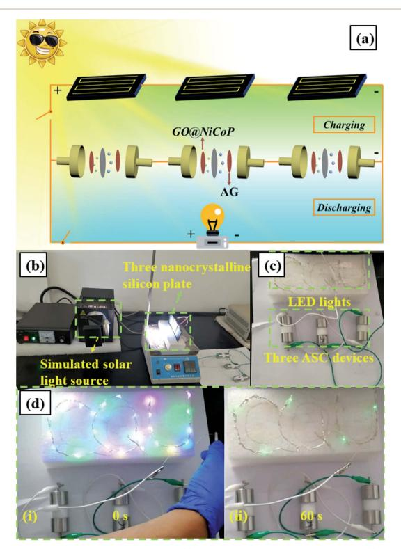
Fig. 8 (a) Schematic illustration of the solar-ECs charging device, (b) the components of the self-charging power station, (c) the LED lights and three ASC devices, (d) lighting 25 LEDs with "CQU" display for about 60 s.
