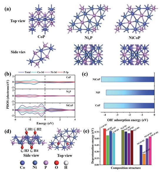
Fig. 6 (a) Top and side views for atomic structures of transition-metal phosphides: CoP, Ni<sub>2</sub>P, and NiCoP, (b) Total and partial density of states calculated for Ni<sub>2</sub>P, CoP and NiCoP systems, (c) adsorption energies of OH<sup>-</sup> on CoP, Ni<sub>2</sub>P, and NiCoP systems, (d) typical representation of NiCoP-OH atomic structure, (e) the calculated deprotonation energy for the deprotonation process on CoP-OH, Ni<sub>2</sub>P-OH, and NiCoP-OH.
