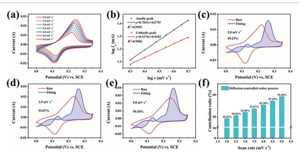
Fig. 5 (a) The CV curves of GO@NiCoP at low scan rates, (b) the plot of  $\log I_p$  versus  $\log v$  for the GO@NiCoP electrode at low scan rates, (c–e) separation of the capacitive and diffusion currents in the GO@NiCoP electrode at a scan rate of 2.5, 3.5 and 5.0 mV s<sup>-1</sup>, respectively, (f) the capacitance ratio of the surface capacitance effect at different scan rates.
