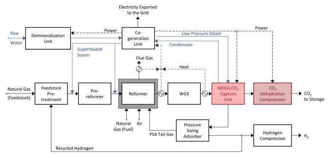
Scheme 3 Hydrogen production via steam methane reforming with MDEA CO<sub>2</sub> capture. The SMR process scheme is adapted to accommodate the addition of the capture unit before the PSA unit. CO<sub>2</sub> is recovered from the shifted syngas, and subsequently dehydrated and compressed to be suitable for geological storage. The raw hydrogen is purified in the PSA unit and the tail gas is burnt in the external furnace, as in Scheme 1.
