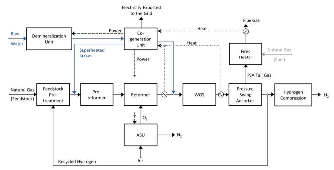
Scheme 2 Hydrogen production via autothermal reforming; to produce high -purity hydrogen an air separation unit (ASU) is needed. On the contrary to the SMR process, the heat required from the process is internally provided. The PSA tail gas in burnt in a fired heater, and the heat originated by the combustion is used to pre-heat some streams
