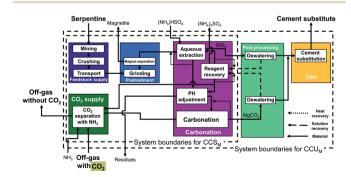
Fig. 7 Process flow diagram of carbon capture and utilization by mineralization via indirect concept of the Nottingham pathway (pH swing) using serpentine. CCS<sub>M</sub> is carbon capture and storage by mineralization. CCU<sub>M</sub> is carbon capture and utilization by mineralization.
