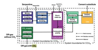
Fig. 4 Process flow diagram of carbon capture and utilization by mineralization via direct mineralization in CSTR using serpentine (pathways CSTR 150 bar and CSTR 10 bar; pathway CSTR 10 bar does not require  $\rm CO_2$  separation).  $\rm CCS_M$  is carbon capture and utilization by mineralization.
