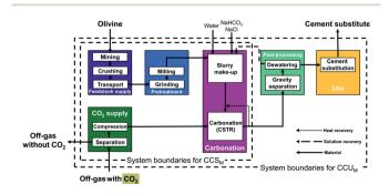
Fig. 3 Process flow diagram of carbon capture and utilization by mineralization via direct mineralization in CSTR using olivine (pathways CSTR 150 bar and CSTR 100 bar).  $CCS_M$  is carbon capture and storage by mineralization.  $CCU_M$  is carbon capture and utilization by mineralization.
