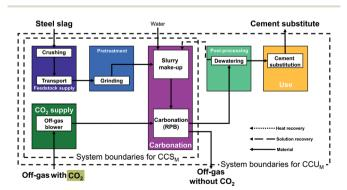
Fig. 5 Process flow diagram of carbon capture and utilization by mineralization via direct mineralization in rotary packed bed reactor (RPB) using steel slag.  $CCS_M$  is carbon capture and storage by mineralization.  $CCU_M$  is carbon capture and utilization by mineralization.
