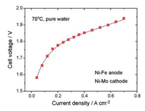
Fig. 3 Cell performance of the first prototype of an AEM water electrolysis system using Ni-Fe anode and Ni-Mo cathode and working only with pure water.33 Reproduced from ref. 33 with permission. Copyright@2014. Royal Society of Chemistry.
