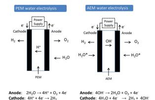
Fig. 1 Comparison of water electrolysis cells and chemistries using either a Proton Exchange Membrane (PEM) or an Anion Exchange Membrane (AEM).\* Current AEM electrolyzers use a water feed with added electrolyte (HCO<sub>3</sub><sup>-</sup>/CO<sub>3</sub><sup>2-</sup> or dilute KOH) to obtain sufficient
