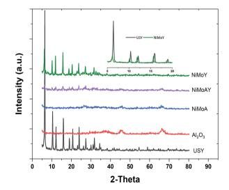
Fig. 6 XRD pattern of the synthesized catalysts, parent USY and  $\gamma$ - $Al_2O_3$
