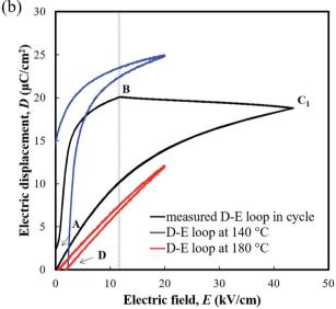
Fig. 5 (a) Temperature dependence of the net mean power of PNZST samples in the laboratory generating assessments.  $\Delta T$  was 40 °C in all ranges; (b) results of the theoretical generating potential evaluation with PNZST samples at  $T_{\rm H}=180$  °C and  $E_{\rm H}=12$  kV cm $^{-1}$ .
