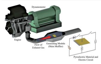
Fig. 2 A schematic diagram of the engine dynamometer assessment (Daihatsu, home-made). The pyroelectric material is set inside the generating module (main muffler).
