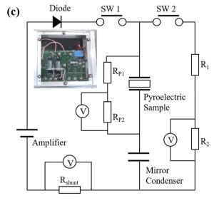
Fig. 1 (a) A schematic of bipolar D–E loops for a pyroelectric material at high and low temperature along with the novel electro-thermodynamic cycle, (b) the cycling conditions for the D–E loop, and (c) a harvesting circuit with a diode and two switches (DSW).
