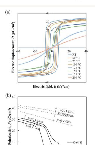
Fig. 4 (a) Hysteresis D–E loops and (b) the polarizations of the PNZST ceramic as a function of temperature.
