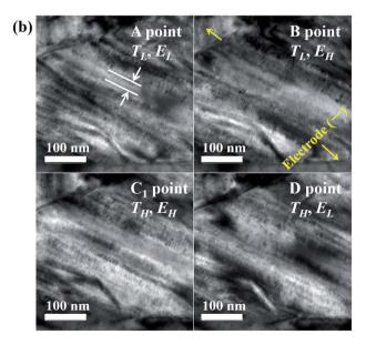
Fig. 3 (a) Refined profiles of a sample at room temperature from the powder using neutron diffraction data and the crystal structure of the *R3c* phase for PNZST, and (b) the microstructures of PNZST ceramics observed by *in situ* transmission electron microscopy (TEM) experiments.
