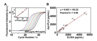
Fig. 3 Performance of the aptamer-assisted proximity ligation assay for N protein detection in human serum. (A) qPCR curves of different concentrations of N protein spiked in 100% human serum. Inset: Linear relationship of  $\Delta$ Ct values and protein concentrations. (B) Comparison of the aptamer-assisted proximity ligation assay with a commercial ELISA kit for N protein detection.
