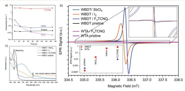
Fig. 6 (a) Time-dependent stability measurements of the conductivity of WBDT with different dopings. (b) EPR spectra of WTA, WBDT and the respective dopings. The insets show a zoom for the undoped spectra and the relative EPR signal intensities. (c) UV-vis-NIR absorption spectra of doped WBDT.
