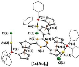
Fig. 2 Molecular structure of homotrinuclear [1c(Au)<sub>3</sub>] with partial atom numbering scheme. Thermal ellipsoids are set at the 50% probability level. For clarity, the phenyl rings are depicted in wireframe style, and co-crystallised solvent, disorder in the P(2)-Au(2)-Cl(2) fragment, and hydrogen atoms have been omitted.
