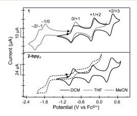
Fig. 4 Solution and solid state cyclic voltammograms of 1 and 2-bpy<sub>s</sub>, respectively, recorded in DCM (solid lines), THF (dotted lines) or MeCN (dashed lines) solutions of TBAPF $_6$  (0.1 M), at a scan rate of 200 mV s $^{-1}$ . The data for 2-bpy $_{\sigma}$  was recorded by dropcasting crystalline material on a glass carbon disk electrode.
