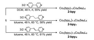
Scheme 2 Self-assembly of van der Waals nanosheets, **2-bpy**, **2-bpy** $_\sigma$  and **2-bpy** $_\pi$ , from tritopic nanoblock 1 and pyridyl-based ditopic linkers.
