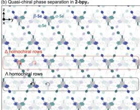
Fig. 2 (a) Single crystal X-ray structure for single layers of 2-bpy, 2-bpy $_{\sigma}$  and 2-bpy $_{\pi}$  (top and side views), illustrating the variations in tile sizes and layer corrugation. (b) In-plane anisotropy and quasi-chiral phase separation in 2-bpy $_{\sigma}$ . Linkers and nanopropeller blades are colored blue when linked to  $\beta$ -Se, and teal when associated with  $\alpha$ -Se sites.
