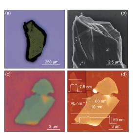
Fig. 5 The laminar structure of 2-bpy $_\sigma$  revealed by imaging pre- and post-mechanical exfoliation of a single crystal. (a) Optical microscopy image of a bulk single crystal. (b) Scanning electron microscopy image focused on laminar edge of the bulk crystal. (c) Optical microscopy of a mechanically exfoliated flake. (d) Atomic force microscopy characterization of the exfoliated flake, including height profiles and a zoomin inset of a thin flake.
