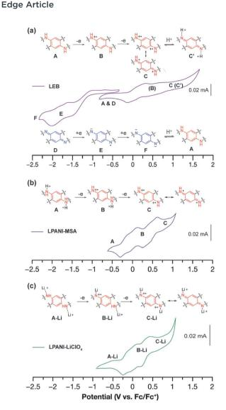
Fig. 3 Cyclic voltammograms of (a) the LEB film in acetonitrile with 0.1 mol L $^{-1}$  TBAPF $_6$ . (b) LPANI solution in THF with 0.15 mol L $^{-1}$  MSA. (c) LPANI solution in THF with 1.2 mol L $^{-1}$  LiClO $_4$ . In all cases, a Pt wire was used as the counter electrode and Ag/AgCl was used as the reference electrode.
