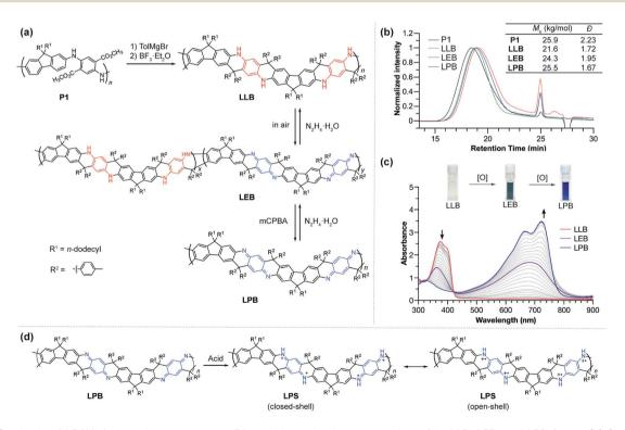
Fig. 1 (a) Synthesis of LPANI from polymer precursor P1, and the redox interconversion of its LLB, LEB, and LPB forms. (b) Size exclusion chromatogram, calculated  $M_{\rm p}$ , and polydispersity ( $\dot{D}$ ) values. (c) UV-vis spectra of the oxidation process from LLB to LEB to LPB in THF; (inset) photographic images of LLB, LEB and LPB solutions. (d) Protonation of LPB with MSA and structural formulae of the closed-shell and open-shell resonance forms of the protonated LPS form.
