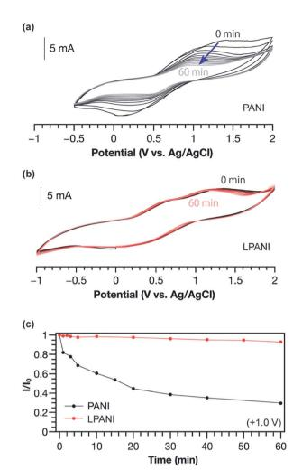
Fig. 4 Cyclic voltammograms of (a) conventional PANI and (b) LPANI after applying +1.0 V potential for a variable amount of time (0–60 min). (c) Plot of the current intensities in (a) and (b) vs. the time of holding at +1.0 V. The experiment was performed on working electrodes (conventional PANI or LPANI solid deposited on carbon fabric cloth) in acetonitrile with 0.5 mol  $\rm L^{-1}$  sulfuric acid. A Pt wire was used as the counter electrode and Ag/AgCl was used as the reference electrode.
