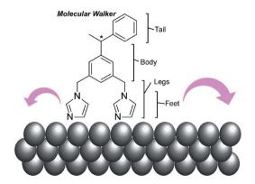
Fig. 5 A chiral molecular walker, 1,3-bis(imidazol-1-ylmethyl)-5(1-phenylethyl)benzene, on a Cu(110) surface.
