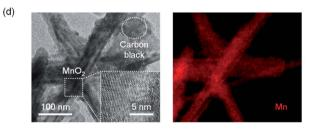
Fig. 4 (a) Cycling performance of a Zn|TpPa-SO<sub>3</sub>Zn<sub>0.5</sub>|MnO<sub>2</sub> cell. (b) Charge/discharge profiles at the 100<sup>th</sup>, 200<sup>th</sup> and 800<sup>th</sup> cycles. (c) SEM image of the Zn metal anode after the 800<sup>th</sup> cycle. (d) TEM (left) and EDS mapping (for Mn; right) images of the MnO<sub>2</sub> cathode after the 800<sup>th</sup> cycle.
