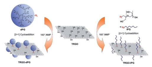
Fig. 6 Schematic representation of inhibitor development by combining thermally reduced graphene oxide (TRGO) with either dendritic polyglycerol (dPG) azide or linear polyglycerol (lPG) azide. Reproduced with permission from ref. 32. Copyright 2017 WILEY-VCH Verlag GmbH & Co. KGaA, Weinheim.
